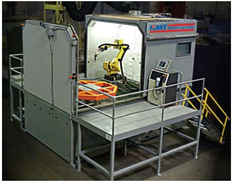
This system is for shell and core removal of large structural parts loaded by crane.
