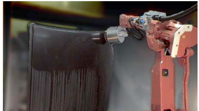
BMW roof being wet ground by KMT RS Robotic System
