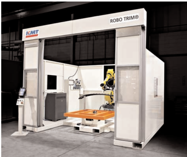
This front view of the RT-500 trimming system shows the riser-mounted AccuTrim™ robot and the servo-controlled rotating table. The RT-500 can trim parts up to 60" x 60" x 36" (1524mm x 1524mm x 94 mm).
