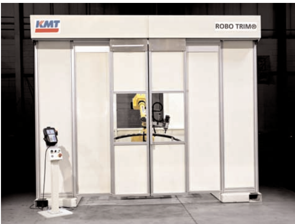
The RT-500 system's steel enclosure with manual front doors protects the operator while the robot is trimming.
