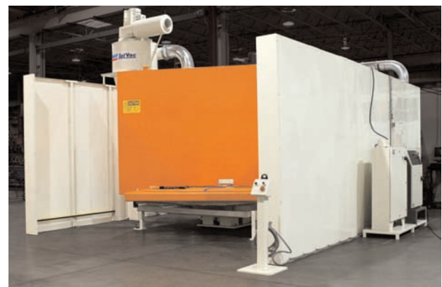
Plastics Unlimited's router trimming system (shown above) is used to trim custom thermoformed products.
