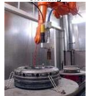
High Pressure Cleaning
